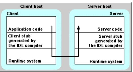
The transmission of service requests and responses between clients and servers is handled by both DCE and CORBA so that applications need not deal with concerns like: where clients and servers are located on the network; differences between hardware platforms, operating systems, and implementation languages (for example, data formats or calling conventions); networking protocols; and others.
