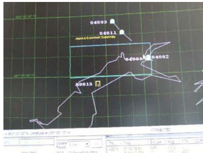
Figures 5 and 6. Close up of the IMTDS display. Shows Air Force aircraft and an ADS-B track; these were forwarded to the cockpit.
