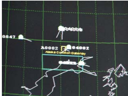
Figure 8. Hangar located IMTDS LINK-16 display, showing one ADS-B and several aircraft.
