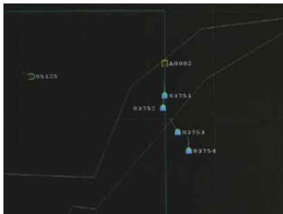
Figure 12. A group of LINK 16 aircraft on “intercept” with our ADS-B control aircraft in flight.
