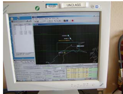
Figures 5 and 6. Close up of the IMTDS display. Shows Air Force aircraft and an ADS-B track; these were forwarded to the cockpit.
