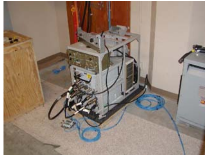
Figures 3 and 4. GBT, Gateway and IMTDS systems, set up. The LINK-16 radio rack.
