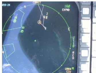
Figure 7. Cockpit shot of the LINK-16 display, ADS-B track in upper right hand corner, ID in lower right hand corner. ADS-B track highlighted and details in lower right corner “unknown civilian.”
