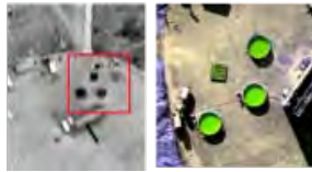
Figure 1: (left) A 10.73 μm grayscale image chip of SEBASS LWIR HSI data showing three water pools. (right) A false-color composite high-resolution context image corresponding to the area in the SEBASS image on the left. The water pools are the three green circular features
