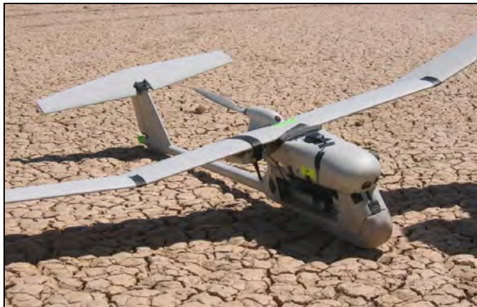
Figure 3. UBR-TX attached to PUMA UAS.
