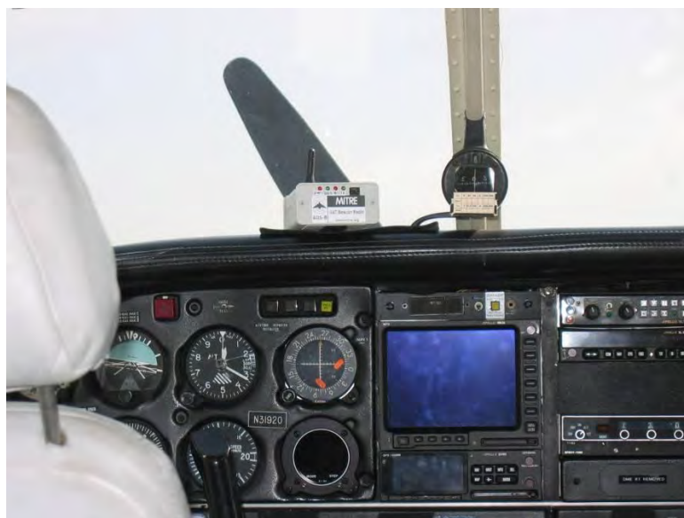
Figure 1. UBR-TX in-place on the glareshield of a piper lance.
