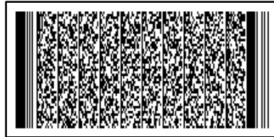
Figure 14-2 Example of 2D Barcode (PDF 417 Type)
