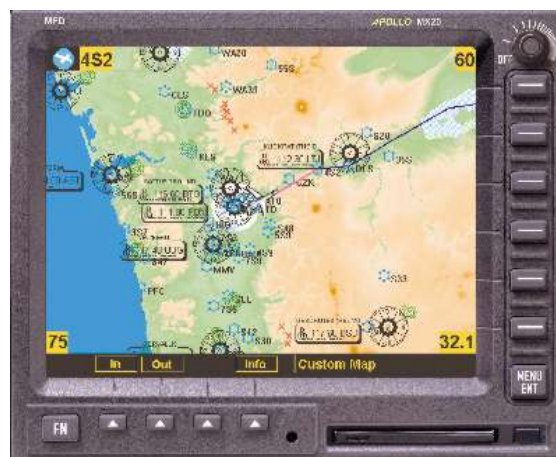
Figure 2.5-3. Garmin MX-20 Multi-Function Display
