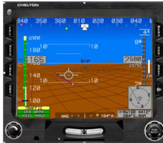
Figure 2.5-1. Chelton EFIS-2000 Primary Flight Display
