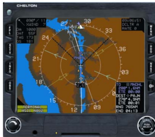
Figure 2.5-2. Chelton Navigation Display
