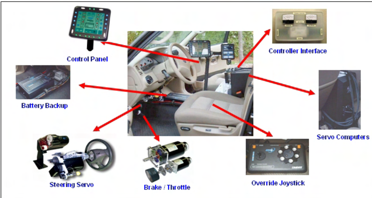
Figure 2: EMC provided the drive-by-wire capability using a steering servo, a throttle/brake servo, a control console, two servo computers, a battery back up, and a manual override.
