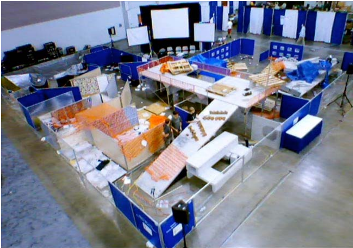
Figure 1. The NIST Reference Test Arena, used in the AAI Robot Rescue Competitions. Shown is an overview photo of the arena from AAI-2004. The orange area is in the foreground with the yellow area to the left and red area to the back right.
