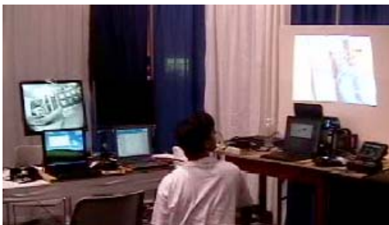
Figure 10. Team H's interface set up in 2004. To the left is the station for operating one of the snakes. The top monitor shows the video from the snake and the two computers are used for control. To the right is the projected video from the other snake, with the RC car's video shown on the computer screen below that. To the right of the computer is the joystick for driving the second snake and the controller for the RC car is to the right of the joystick. The operator would move back and forth between the two stations.
