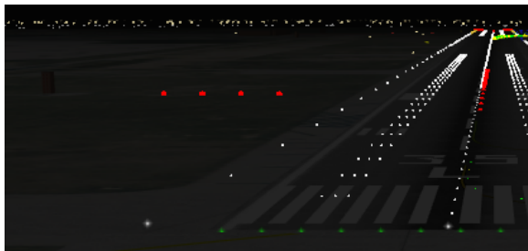
Arrival Occupancy Lights from the Cockpit
