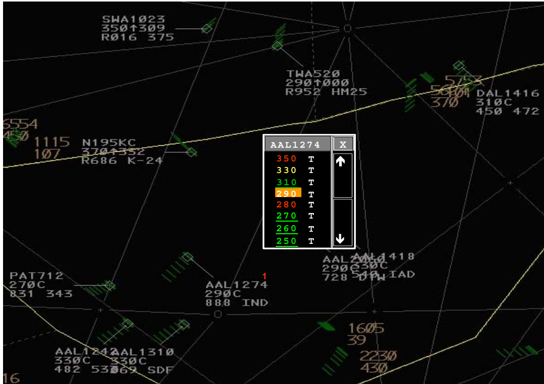
Figure 4-2. Notional Integrated Sector Operation Display
