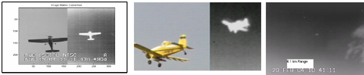
Figure 3-8. The detection of single engine Cessna (left), a crop duster (middle) and a twin engine Cessna at 6.1 km (right)
