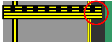
Extension past taxiway edge markings
