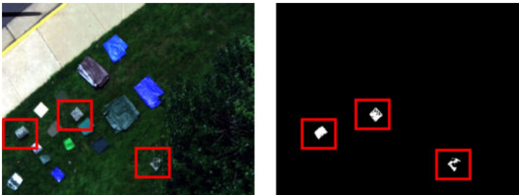
Figure A-3: (Left)RGB from cube 2018-07-27_15_46_10. (Right)Camo detection on cube 2018-07-27_15_46_10 using signature from same cube.
